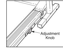
knob counterclockwise. To decrease the firmness, turn the knob clockwise. Note: The faster you run on the treadmill, or the more you weigh, the firmer the cushioning system should be.
